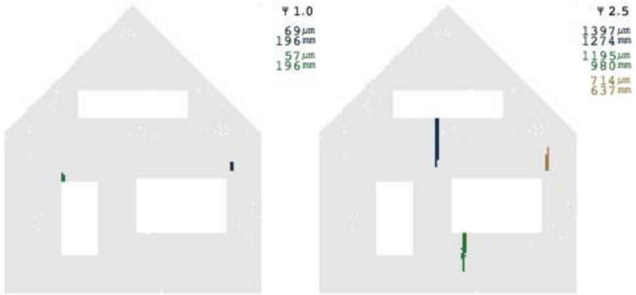
Figure 3.16. Crack pattern of Façade 4, geometry A, standard material, soil A, original interface and asymmetric settlement, knick point=L/3. Cracks at DS1 (left) and DS2 (right). Notice how new cracks allow other cracks to close.
