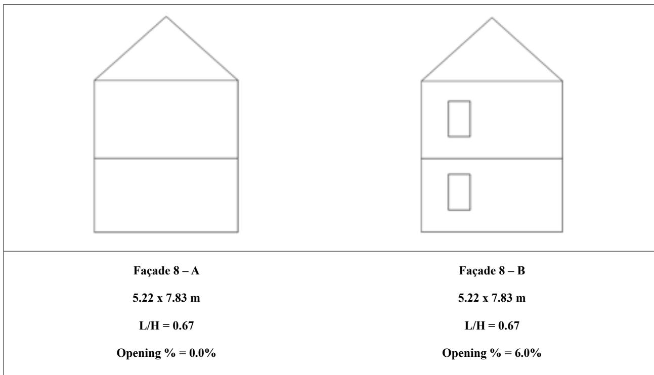
Figure 2.19. Two geometry variations of Façade 8.
