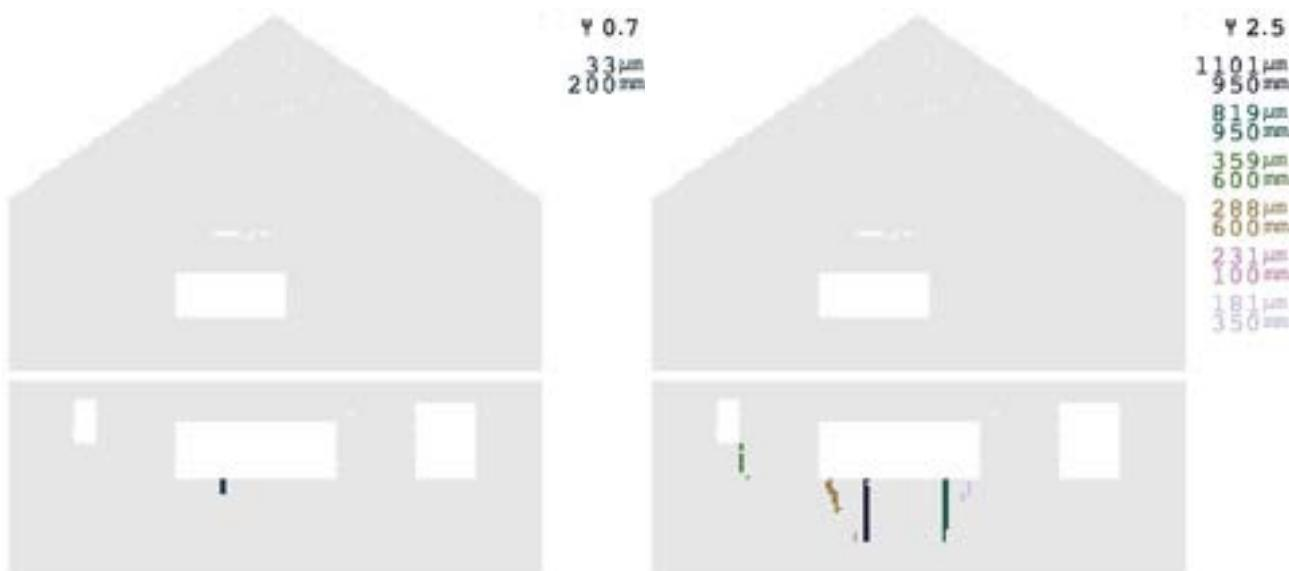
Figure 3.28. Crack pattern of Façade 6, geometry A, standard material, soil A, original interface and asymmetric settlement, knick point=L/3. Cracks at DS1 (left) and DS2 (right).
