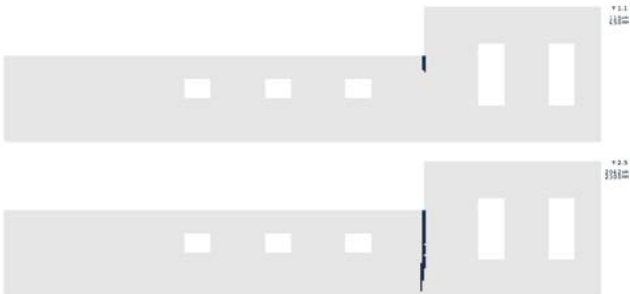
**Figure 3.14. Crack pattern of Façade 2, geometry A, standard material, soil A, original interface and symmetric settlement, knick point= $L/2$ . Cracks at DS1 (top) and DS2 (bottom).**
